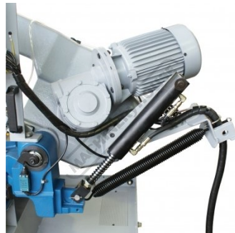
Motor and Gearbox Drive
