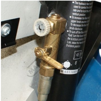
Down Feed Control
